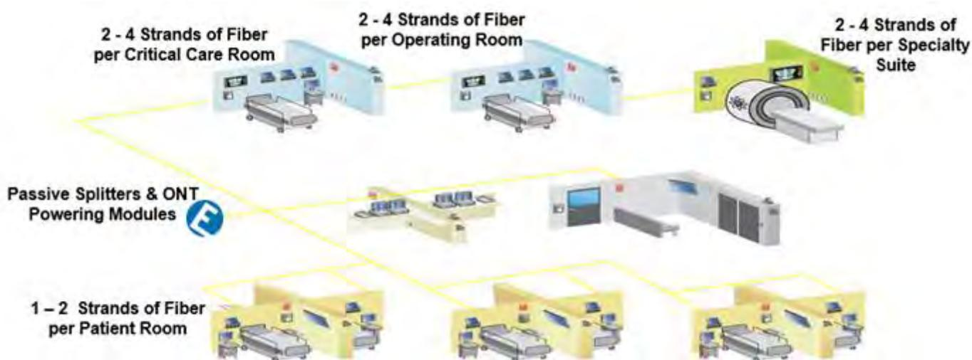
**Figure #2:** Fiber based Tellabs Optical LAN and converged network architecture
